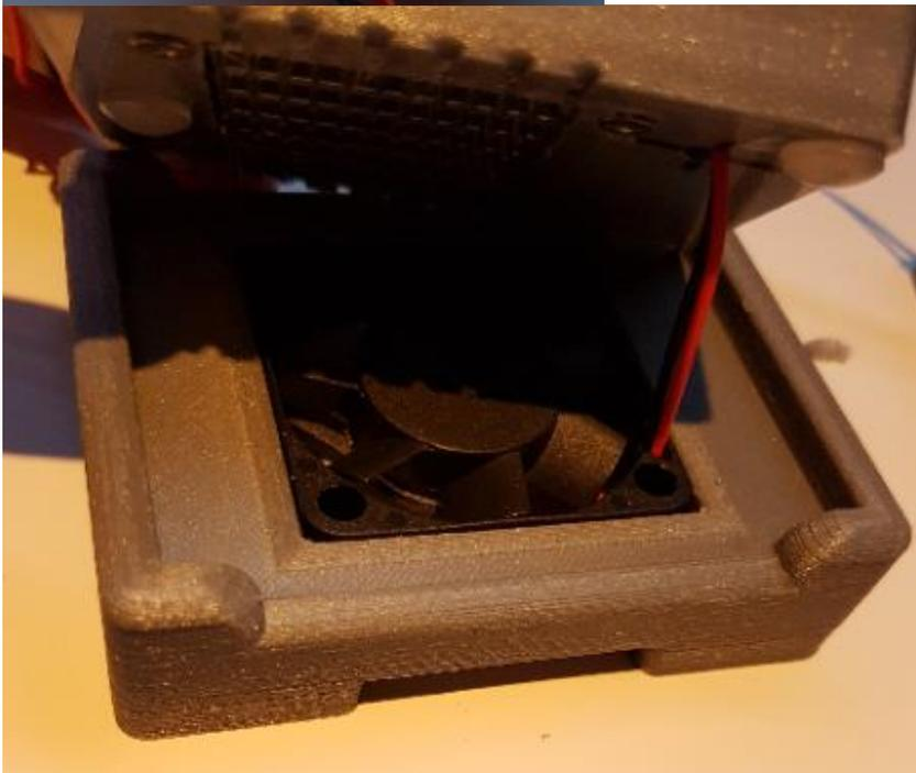
Also note that the wires from the fan are on the same side as the hole you just drilled.
